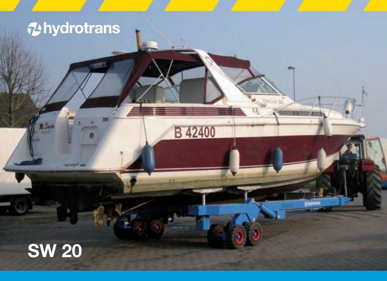
The Hydrotrans SW20 slipway trailer is also suitable for transporting boats on T-cradle's. The solid or pneumatic tires of the SW20 offers optimal security through any terrain capable of carrying the load.
