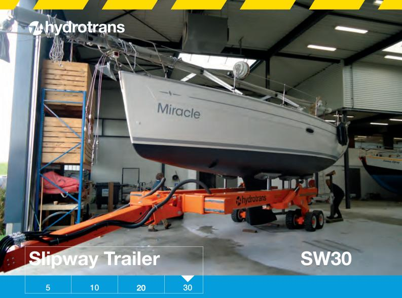
The Hydrotrans hydraulic boat trailer is designed to launch and recover boats on a slipway, transport the boats over land and park them in a storage or work area.
