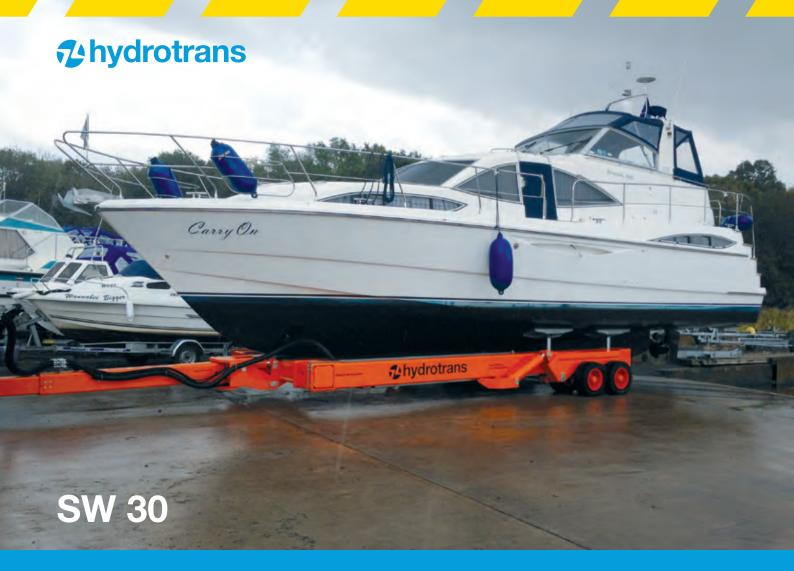
The Hydrotrans SW30 slipway trailer is also suitable for transporting boats on T-cradle's. The solid or pneumatic tires of the SW30 offers a comfortable ride through any terrain capable of carrying the load.
